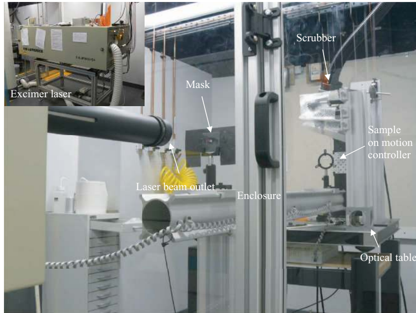
FIG. 1. A typical ELAP setup for treatment of Ag-TiO 2 thin films, inset shows the GSI excimer laser system.
