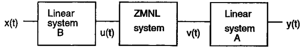
FIGURE 1 Generalized system using linear functions in series with a zero memory nonlinear function.
