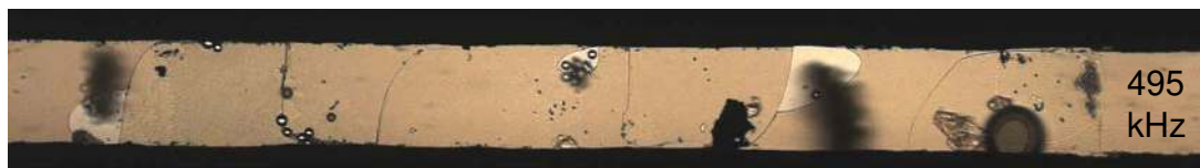
Figure 8.10: Shattered silicon-nitride membrane due to the high amplitude mechanical vibrations coupled from the silicon. This particular case occurred at 495 kHz with few volts peak to peak drive where a resonance of the whole pzt-silicon actuator exist.
