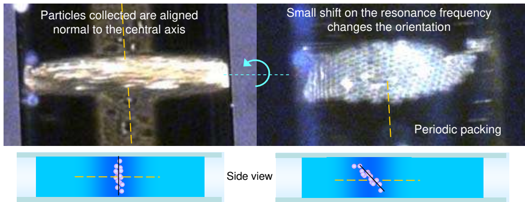
Figure 8.17: After particles are collected at a pressure node, their alignment with the central axis can be changed by a slight frequency shift. This alignment change reveals the crystalline packing structure of the particles collected under acoustic radiation pressure forces.
