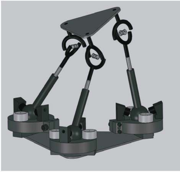
Figure 4. Under-actuated manipulator with topology 3-nSPU: (a) kinematic model, (b) 3D CAD model of a manufacturing scheme.
