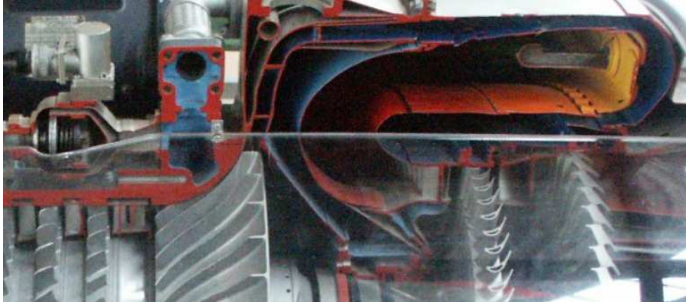
Figure 9.3 Reverse flow combustor gas turbine configuration
