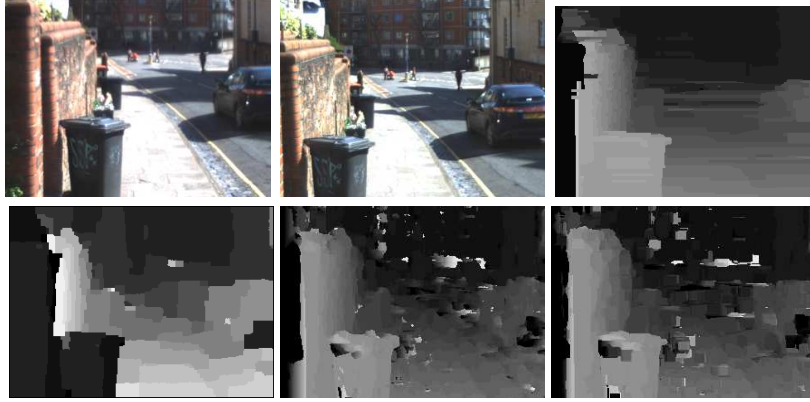
Figure 2: 1st row: stereo images and depth estimation based on dynamic programming using 1D optimisation; 2nd row: results obtained from belief propagation, sum of absolute differences with winner-take-all optimisation, and sum of squared differences with iterative aggregation.
