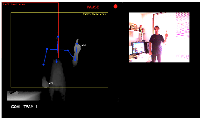
Fig. 4. Static and dynamic gesture recognition prototype interface.
