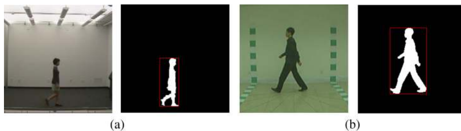
Fig. 2 Results of foreground segmentation and preprocessing on sample sequences from (a) Georgia Tech (GT) and (b) CASIA datasets.
