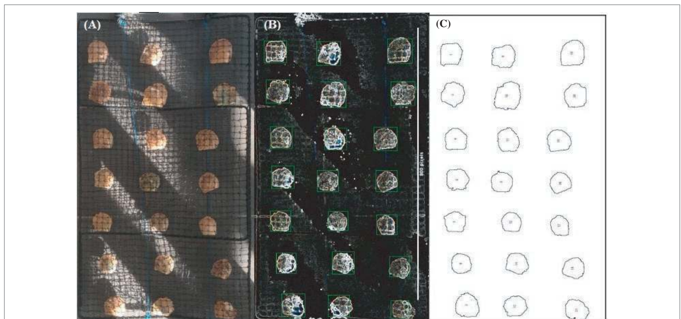
FIGURE 3 | Different stages of predicting pearl oyster size through MVS and machine learning algorithm. Pearl oysters in net are placed on a table while being cleaned, and visual image is taken from above. (A) Oyster net image depicts one of the most challenging visual capture situations in pearl oyster commercial environment. (B) Oysters and net have low contrast from the background, and lighting is variable. (C) Sliding window CNNs correctly identified and measured oyster size with >96% accuracy. (Photo image by Preston Toole).
