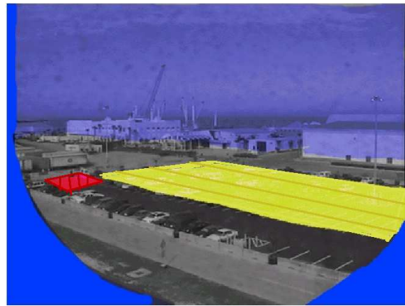
Figure 4. An alarm map associates rules with pixels in the image. The red (small vertically striped region on left) has rules that activated only for cars leaving (not entering) off-hours. The yellow (lighter region in parking lot) has rules that alarm for people-sized targets anytime. The yellow region hands-off to a PTZ so a guard can assess what the human is doing. The blue regions (sky and lower corners) are ignored. The remaining regions will detect/track targets but do not set off alarms.
