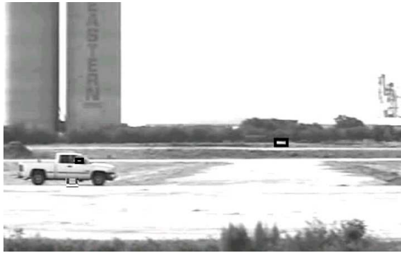
Figure 3. As is well known, distant targets appear smaller than near-by targets. The feet of the person behind the truck have more pixels than the backhoe in the distance. The perspective effect makes image-based rules difficult to apply in filtering nuisance alarms.
