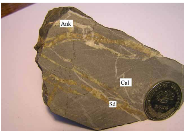
Figure 9: Brown siderite and pale yellow ankerite veins and tiny white calcite veinlets that cut the studied limestone (sample TVAP1).
