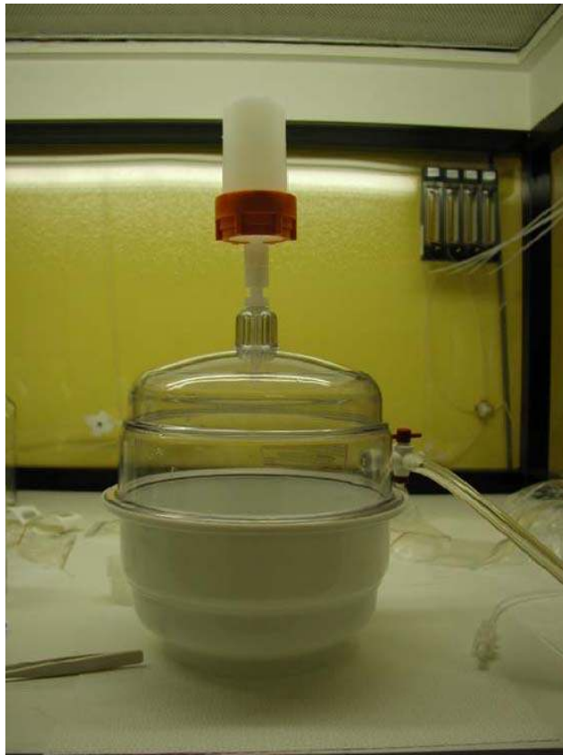
Figure 10: Vacuum-desiccator filtration chamber with filtration assembly attached (Photograph by Michael E. Lewis, after F. Wilde, et al. 2004-2009(b))
