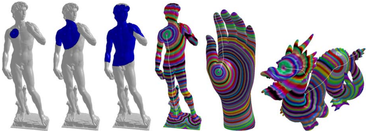
Figure 2. Front Propagation (on the left), level sets of the distance function and geodesic paths (on the right).
