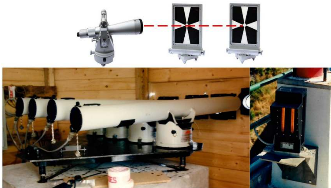
Figure 1. Evolution of collimators from purely manual instruments (on the top) to opto-electronic automatic systems (on the bottom: ISAC 5000 by ISMES S.p.a., Seriate, Italy).
