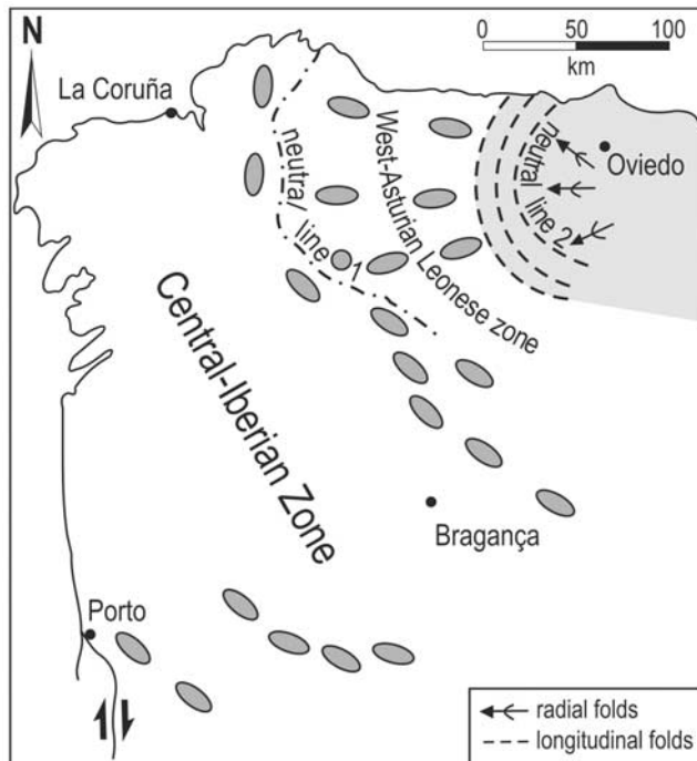
Figure 12. Deformation and internal strain in the Ibero-Armorican Arc. Structures developed during the thick-skinned stage involved longitudinal stretching in “b” kinematics axis, neutral line 1, with pure flattening and radical stretching in “a” kinematics axis. Structures developed during the thin-skinned stage are restricted to the Cantabrian Zone, with longitudinal folds, neutral line 2, and radial folds. Data are from Ribeiro [1974], Matte and Ribeiro [1975], Pérez-Estaún et al. [1980], Ribeiro et al. [2003], and Gutiérrez-Alonso et al. [2004].
