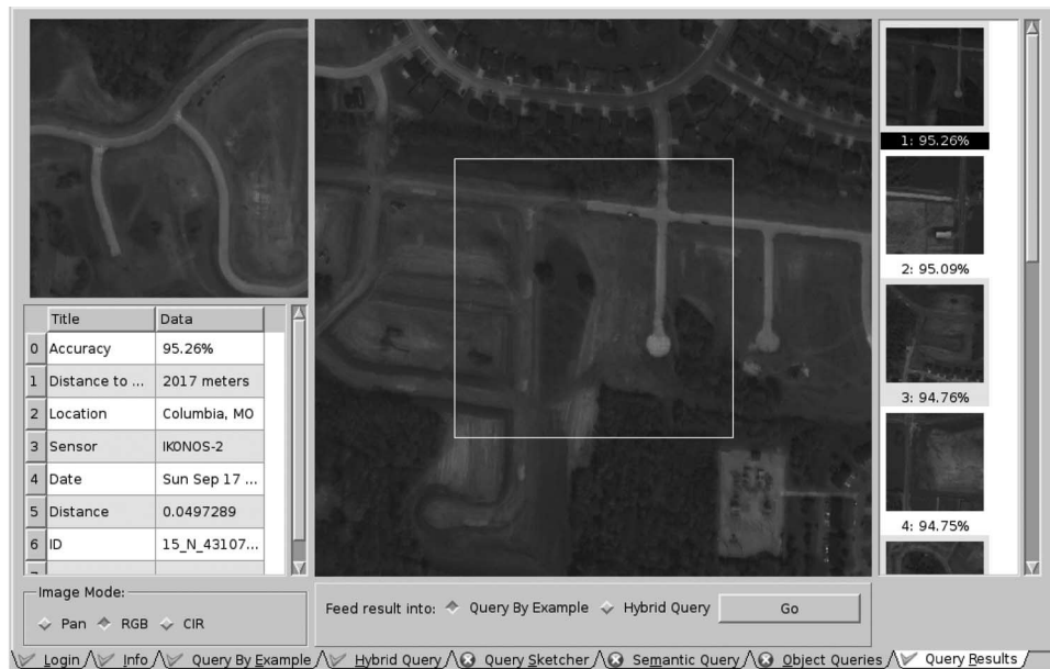
Fig. 10. Hybrid query results visualization of construction within 3 km of a school. The query image is shown in the upper left-hand corner. The current result is shown in the large center image, and the associated metadata are shown in the lower left-hand corner. A ranked list of the top relevant results is shown on the right.
