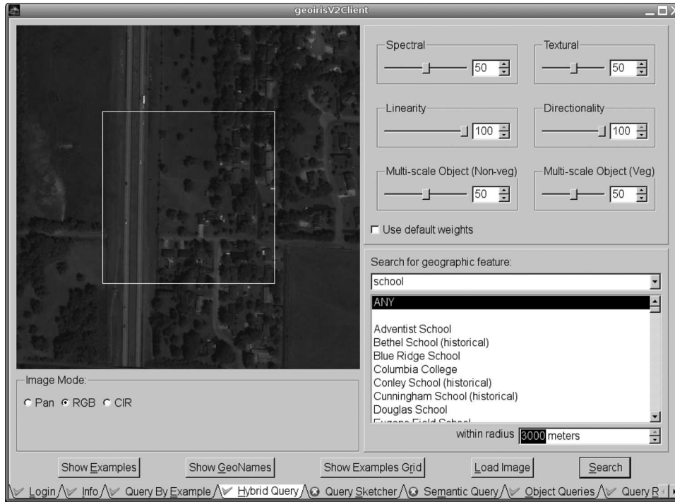
Fig. 9. Example of a hybrid query being built. The query image is the region of interest within the white rectangle (i.e., the divided highway). Weights can be assigned to features of various indexes by adjusting the sliders, and the use of heterogeneous databases is demonstrated by specifying the constraint that results must be within 3 km of a school.
