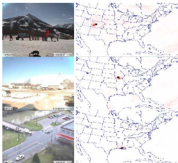
Figure 1. It is possible to geolocate an outdoor camera using natural scene variations, even when no recognizable features are visible. (left) Example images from three of the 538 static webcams that have been logged over the last year. (right) Correlation maps with satellite imagery; a measure of the temporal similarity of the camera variations to satellite pixel variations is color coded in red. The cross shows the maximum correlation point, the star shows the known GPS coordinate.
