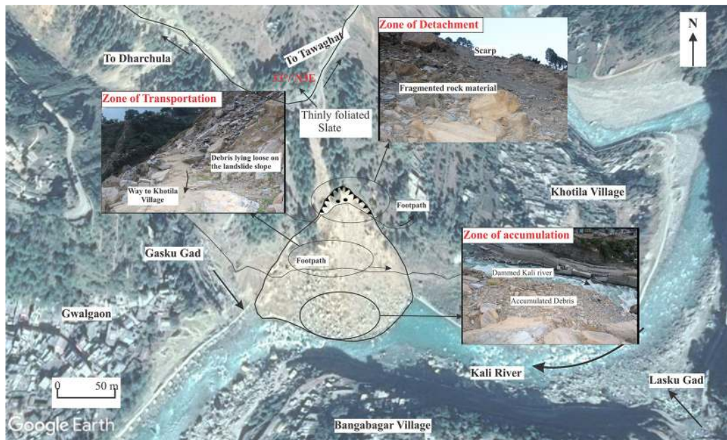
Figure 6. Google Earth image of the Khotila landslide with inset pictures indicating (a) zone of detachment, (b) zone of transportation and (c) zone of accumulation. Black dots represent the location of the soil samples.
