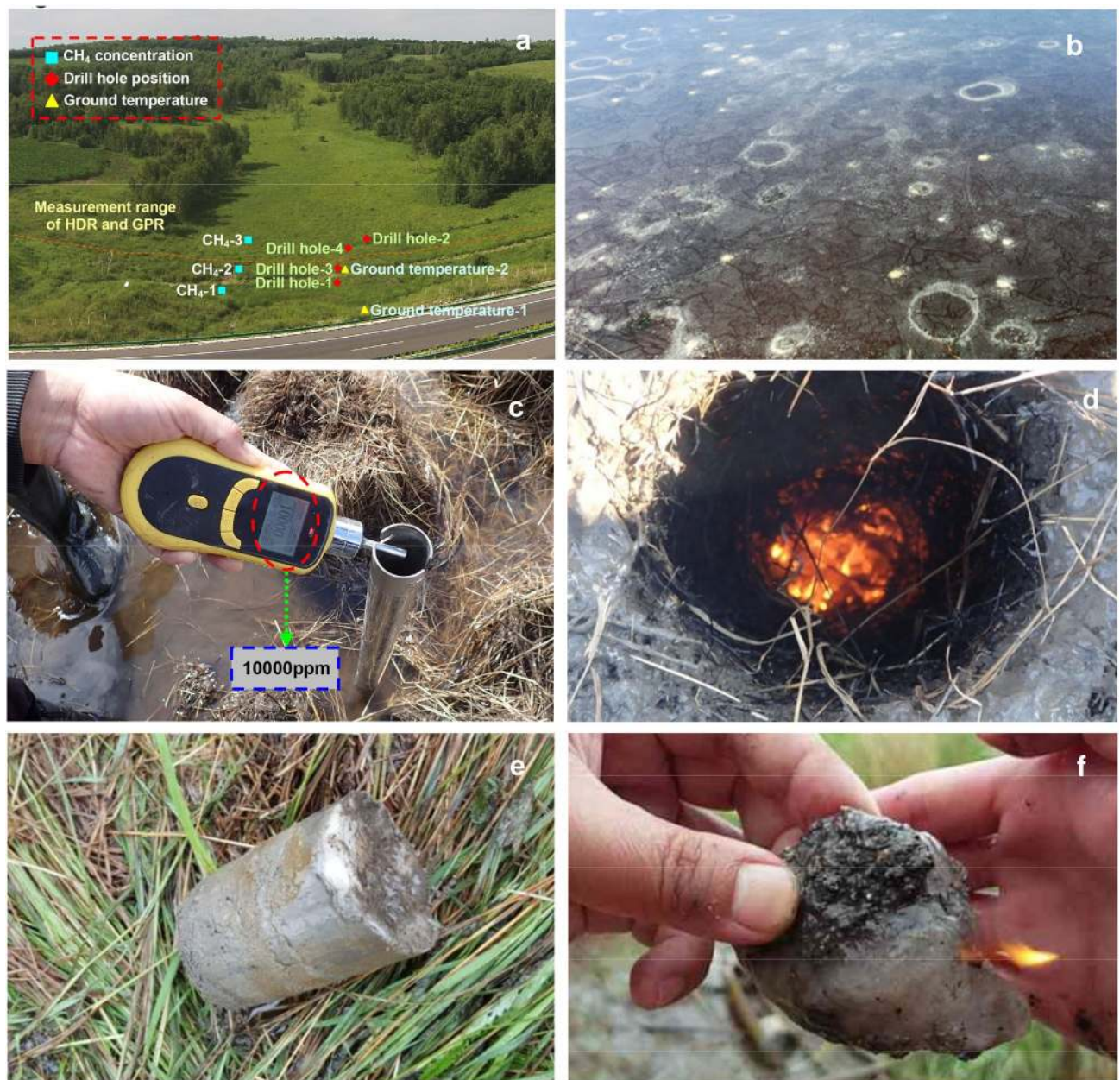
Figure 4. Drilling results and combustible ice samples in study area R-1. (a) Location of the drill hole, the surface methane concentration sensor, the ground temperature sensor, and the measurement range of the high-density electrical method (HDR) and the ground-penetrating radar (GPR) in the study area R-1, (b) High-concentration methane bubbles under the ice surface at the drilling site in spring, (c) High-concentration methane gas discharged along the drill pipe as found by a light drilling machine near borehole 4 (up to 10,000 ppm measuring instrument upper limit; the measuring instrument is an SKZ1050-CH4 methane detector), (d) The flame formed in contact with a fire source after a hole was drilled at a depth of 15 m, (e) Combustible ice samples obtained by drilling 8 m underground at drill holes-3, (f) The burning process of Combustible ice samples on site.
