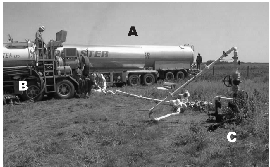
Figure 7 Carbon dioxide injection test into a coal bed, central Alberta, 1998. A =CO 2 cisterns, B = compressor and C = injection well (courtesy of Bernice Kadatz, Alberta Research Council).
