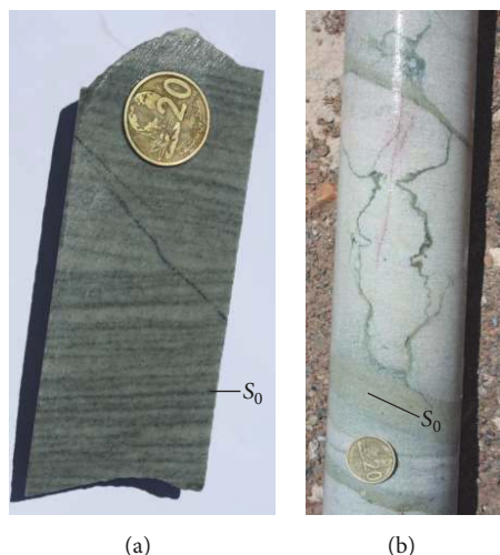
FIGURE 10: Drill core photos showing (a) bedding parallel disseminated mineralization and fracture-hosted copper mineralization and (b) copper sulphides (chalcocite and bornite) along carbonaceous stylolites. S_0 bedding.
