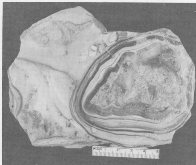
FIGURE 7.—Nodular fluorite consisting of brecciated, silicified rhyolitic welded tuff, chalcedony, and early fluorite surrounded by thin layers of gray and white fluorite; Colorado-American deposit. Scale shown in centimeters. Photograph by J. A. Denson.
