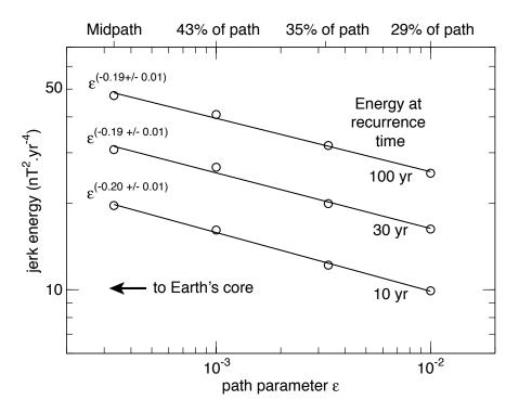
Supplementary Figure 2: Scaling of jerk energy along the parameter space path. Evolution of jerk energy at recurrence times 10, 30 and 100 years, as extracted from Fig. 4b, with the path parameter  $\epsilon$  (Methods and Supplementary Table 1).
