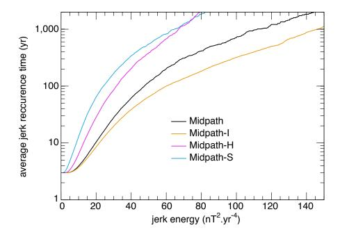
Supplementary Figure 3: Sensitivity of the jerk recurrence time distribution to physical conditions in the lower mantle and upper outer core. Distribution of the average recurrence time of jerks reaching or exceeding a given energy (same as Fig. 4b), for the models Midpath-I and Midpath-H with variable lower mantle electrical conductance, and model Midpath-S with a stratified region in the upper outer core (Methods). The Midpath model result from Fig. 4b is also reproduced for reference.
