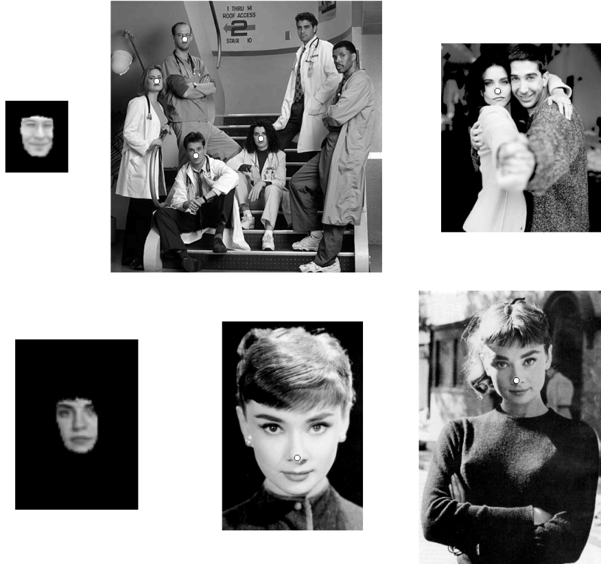
Figure 9: Face detection results. The two leftmost images are masked templates. The white circles in the other images represent the best matches using geometric blur. The templates were compared with each of the images at a range of scales (differing by a factor of 1.4). The white circles represent the matches above threshold at any scale. A single threshold per template is appropriate for detecting faces across multiple images using these templates, indicating good discriminative ability. Either template individually can produce the detection results shown for all four images, indicating good generalization.
