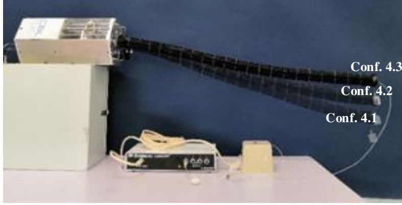
Fig.14 Physical demonstration of the stiffness adjustment under 100g end load
