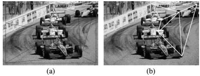
Fig. 15 Content authentication under malicious tampering+incidental modification (JPEG with a quality factor of 30%): a the modified image and its detected meshes; b the areas that were detected as having been maliciously tampered with are indicated by meshes with white lines
