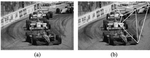
Fig. 13 Content authentication under malicious tampering: a the image modified through object substitution applied to the top-right part of Fig. 11 b ; b the areas that were detected as having been maliciously tampered with are indicated by meshes with white lines
