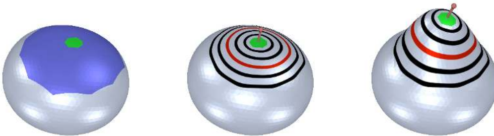
Figure 41: After specifying the blue support region and the green handle regions (left), a smooth scalar field is constructed that is 1 at the handle and 0 outside the support (center). This scalar field is used to propagate and damp the handle's transformation (right).
