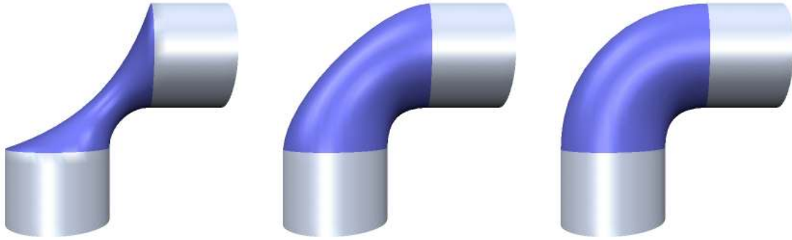
Figure 25: The order k of the energy functional and of the corresponding Euler-Lagrange PDE \Delta_S^k \mathbf{x} = 0 defines the stiffness of the surface in the support region and the maximum smoothness C^{k-1} of the boundary conditions. From left to right: membrane surface ( k = 1 ), thin-plate surface ( k = 2 ), minimum variation surface ( k = 3 ).
