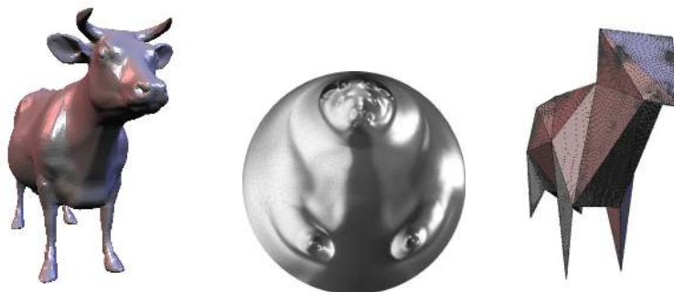
Figure 30: Mapping a cow model (left) to the sphere (center, using [ZRS06]) and to a base triangulation (right, following [LSS*98]). The maps are visualized by the original shading and original vertices in coarse base triangles, respectively.
