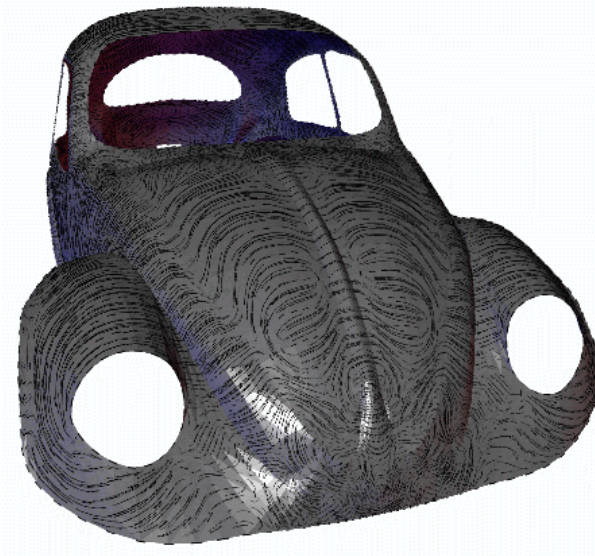
Figure 21: Lines of curvature. Lines of curvature are superimposed on a flat shaded image of a VW Beetle model.
