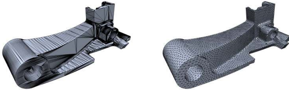
Figure 36: Isotropic, feature sensitive remeshing of a CAD model.
