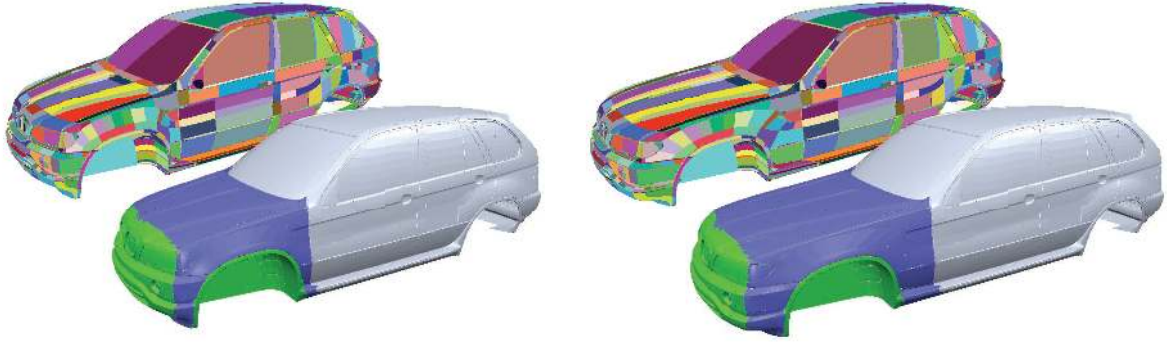
Figure 46: Using multiple independent handle components allows to stretch the hood while rigidly preserving the shape of the wheel houses. This 3M triangle model consists of 10k individual connected components, which are neither two-manifold nor consistently oriented.
