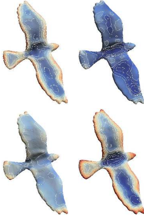
Figure 3.6: illustration of maximum principal curvature \kappa_1 and the minimum principal curvature \kappa_2 in the upper row, and Gaussian curvature K and mean curvature H in the lower row.
