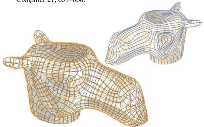
Figure 17: Circular mesh generated by optimizing a mesh generated from principal curves (top right).
