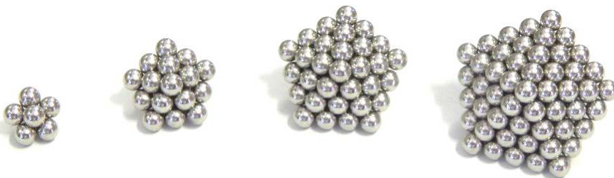
Figure 3. Pentagonal bipyramids with increasing particle numbers. The complete structures number 7, 23, 54, 105 particles. The particle numbers of such structures have nothing in common with nuclear structures, except for the case of some structures of 4-fold symmetry.
