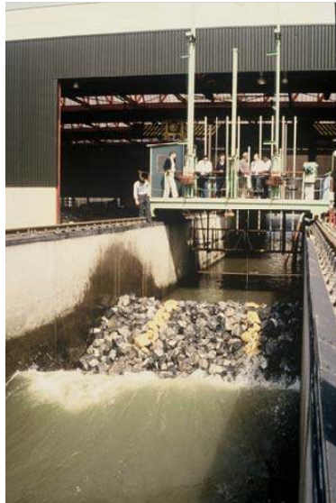
Figure 6. Testing a fully reshaping berm breakwater in the Deltaflume (Courtesy Deltares).
