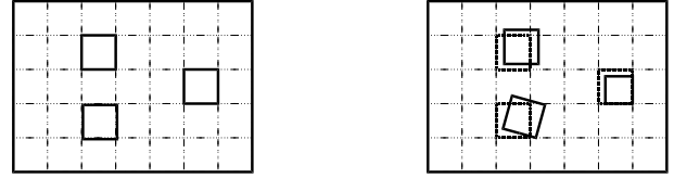
Fig. 4. On the left: the marked image is divided in blocks, the detection of the mark is performed on each block. On the right: several windows generated by the 4-parameter correlation.
