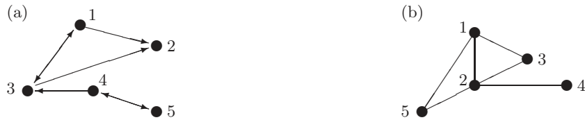
Figure 2.1: (a) A directed graph on 5 vertices. (b) An undirected graph on 5 vertices.
