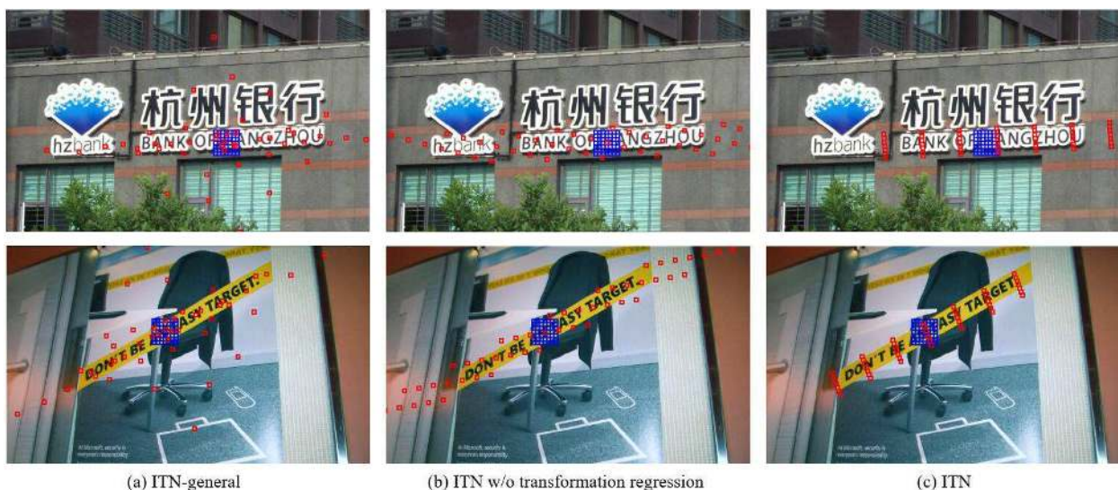
Figure 6. Example of the learnt transformations. Transformed sampling grids (red) and corresponding regular sampling grids (blue) on feature maps (visualized as input images) of (a) ITN-general, (b) ITN w/o transformation regression and (c) ITN.
