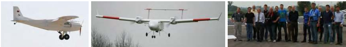
Figure 1. Different platforms used at the DLR Robotics and Mechatronics Center range from regular model aircrafts such as Frauke to the 25kg aircraft ELWIRA. The core team operating these aircraft includes about ten people.
