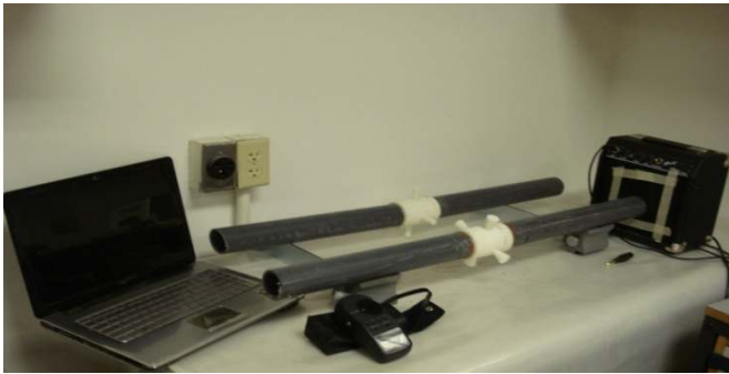
Figure 12: A picture of the experimental setup established to measure the noise attenuation offered by the modeled resonators.
