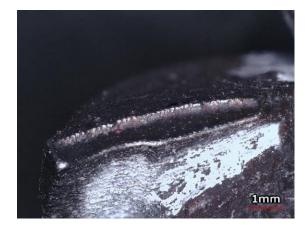
Figure 10. Rounded cutting edge of the as-fabricated tool.
