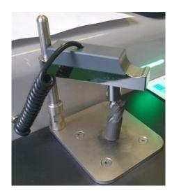
Figure 4. Chemical composition analysis of the printed tool.
