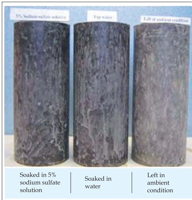
Figure 5. Visual Appearance of Heat-cured Geopolymer Concrete Specimens after One Year of Exposure [12]
