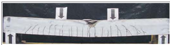
Figure 9. Crack Pattern and Failure Mode of Reinforced Geopolymer Concrete Beam [13]
