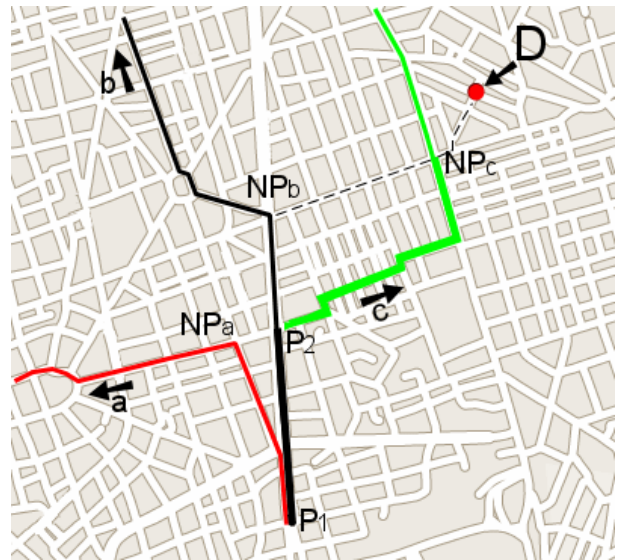
Figure 1: Example of calculation of the Nearest Point (NP) from packet's Destination (D).
