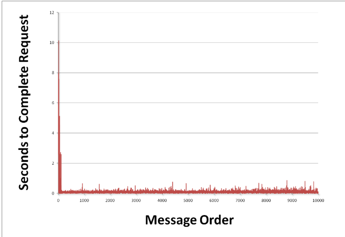
Figure 14. Performance Results of Social Strength Requests that Were Computed Using Direct Remote Peers or Completely Locally.
