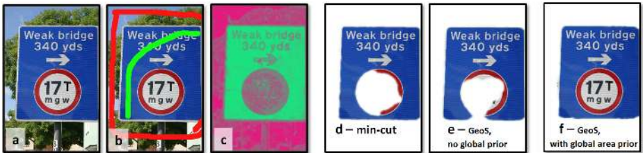
Fig. 9. Exploiting global constraints. (a) Original test image; (b) user provided F_g and B_g strokes; (c) corresponding unaries; (d) min-cut segmentation with \kappa = 0 ; The circular traffic sign is missed out. (e) GeoS segmentation on same energy as in (d); (f) GeoS segmentation on energy with global constraint G = |Area_{F_g}/Area - 0.7| .
