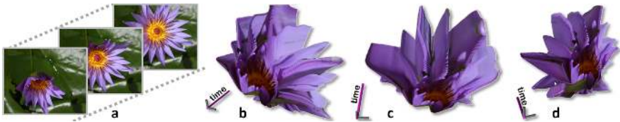
Fig. 10. Batch, space-time segmentation of video. (a) Three frames of a time-lapse video of a growing flower. (b, c, d) Three views of the segmented “video-cube”. GeoS segmentation is achieved directly in the space-time volume of the video.
