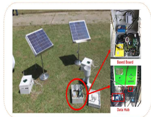
Figure 6. The sensor web with GPRS and Solar Power
