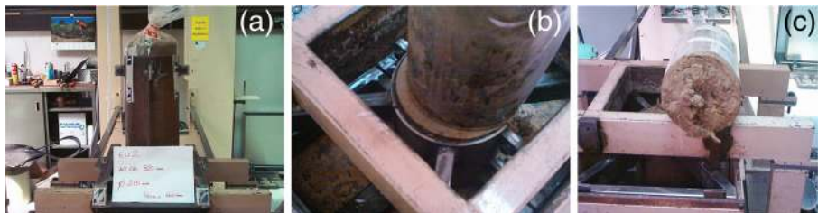
Fig. 14 Direct shear test device. a Positioning of the rooted soil sample inside the steel support. b Direct shear test carried out on the rooted specimen. c Specimen of rooted soil at the end of a direct shear test [57]
