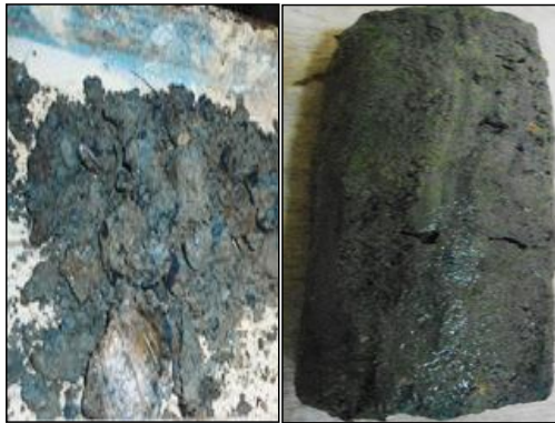
Fig. 5: Soil sample NA10 after extraction from Shelby tube.
