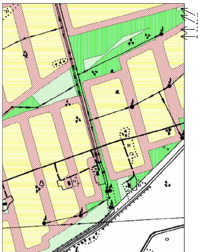
Fig. 6. Layout of mined land in Kohtla. Legend: 1 is steady land, 2 – stable land, 3 – quasistable land, 4 – subsidized land
