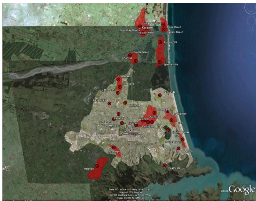
Figure 4.3: Areas of observed liquefaction (red shaded regions and red points) in Christchurch due to the 2010 Darfield earthquake (the liquefaction map is based on surface manifestation of liquefaction visible in aerial photographs and compiled evidence from ground surveying).
