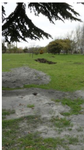
Figure 6.19: Photos 19-20: Lateral spreading cracks along the landside of the stopbank on the north side of the Kaiapoi River. The locations of these photographs are denoted in Figure 6.2. (43.384633°S, 172.661231°E).
