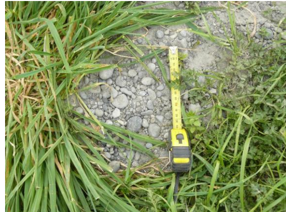
Figure 4.43: Ejected sand and gravel in the Clearwater area (photo by Ian McCahon).
