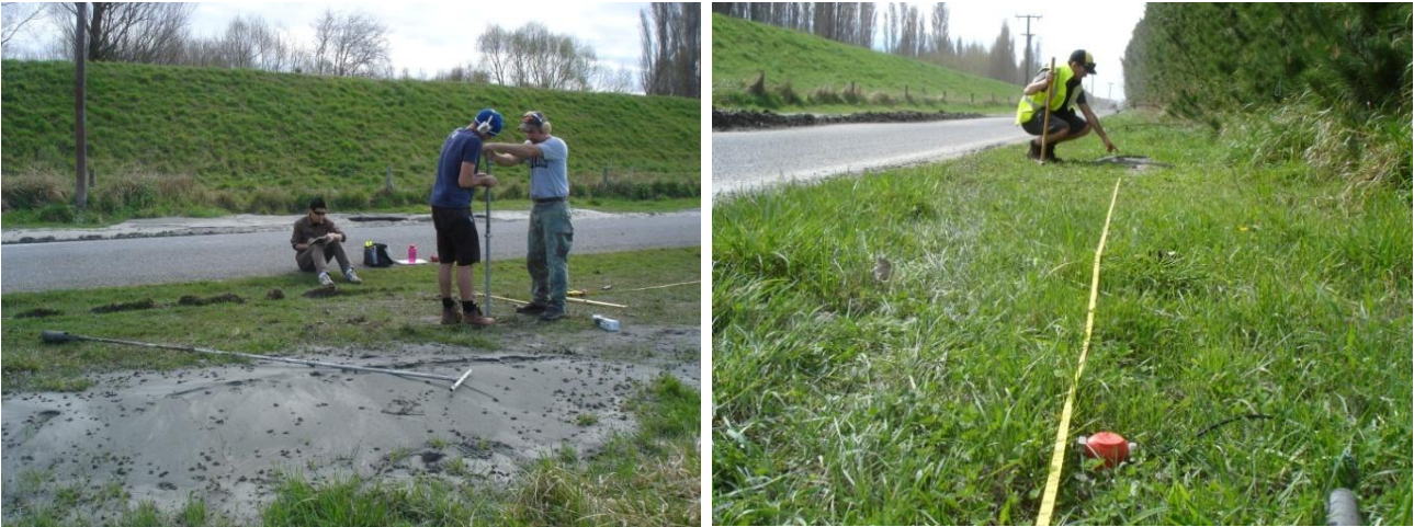
Figure 6.11: Photos 7 and 8: DCPT (left: 43.425137°S, 172.628619°E) and SASW test (right: 43.424342°S, 172.630473°E) performed in areas that did and did not liquefy along the stopbank on Couatts Island Rd .
