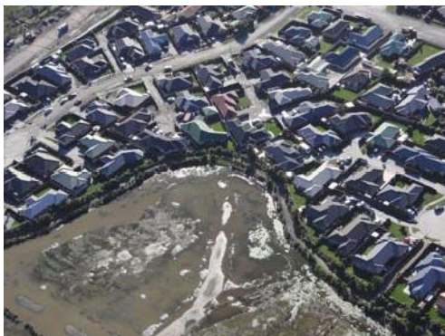
(a) Aerial view of the southern edge of Bexley which was severely affected by liquefaction and lateral spreading; (b) Evidence of liquefaction in residential area (Seabreeze CI).
