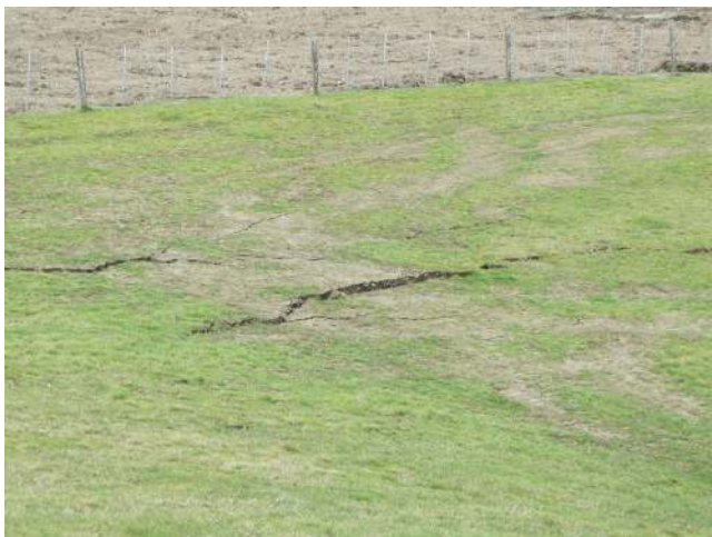
Figure 7.25: Evidence of liquefaction adjacent to Chaney's Overpass.
