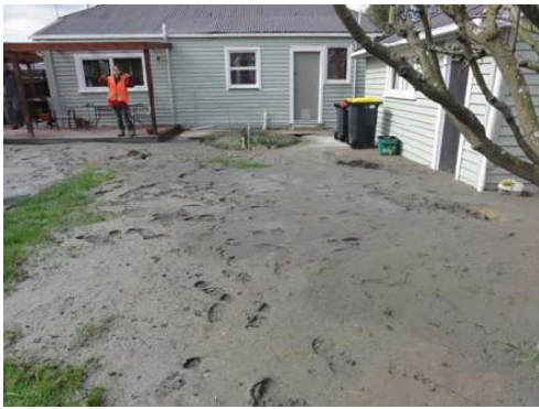
(a) Large sand boils in residential area of Avonside (Bracken St).
