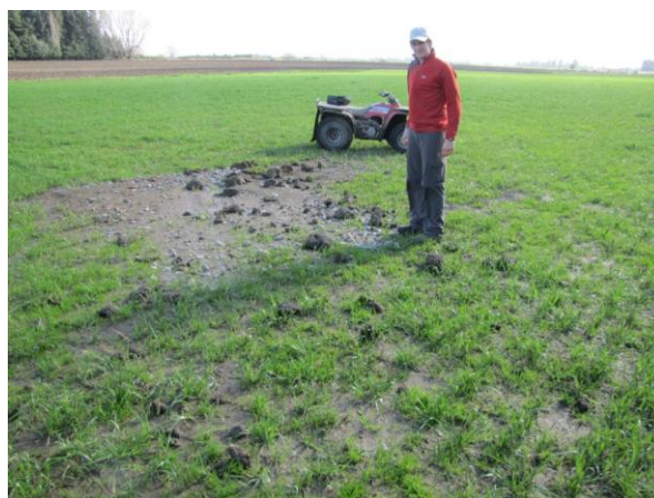
Figure 4.40: Ejected material on another paddock of the Selwyn Forks farm (Sheepyard paddock). As well as sand and gravel the ejecta contain clods of topsoil. (Position marked as Photo 4 in Fig. 4.36).
