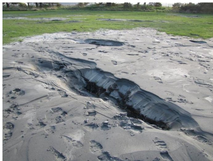
Figure 4.14: Sandboil in the Featherstone Reserve Pines Beach from which sand was taken for electron microscope pictures.
