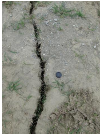
Figure 4.42: Ejected sand and gravel at the Willow Lea property (position marked as Photo 5 in Fig. 4.41).
