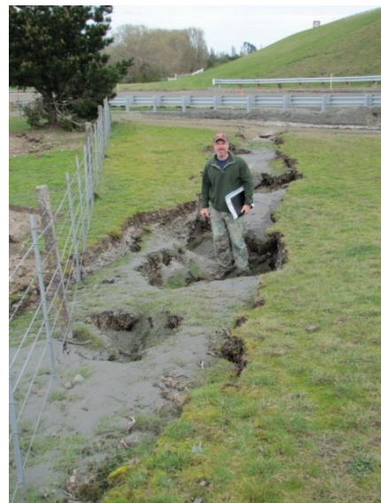
Figure 7.25: Evidence of liquefaction adjacent to Chaney's Overpass.
