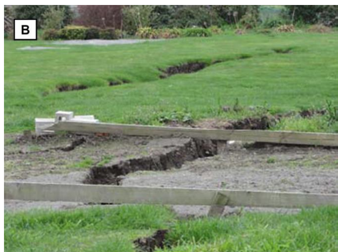
(b) Large lateral spread cracks in farm land (at B: 43.3941389°S, 172.659750°E).
