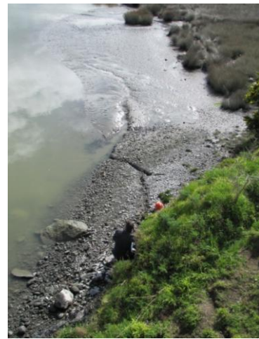
Figure 7.3: Lateral spreading of east banks adjacent to the Bridge Street Bridge.
