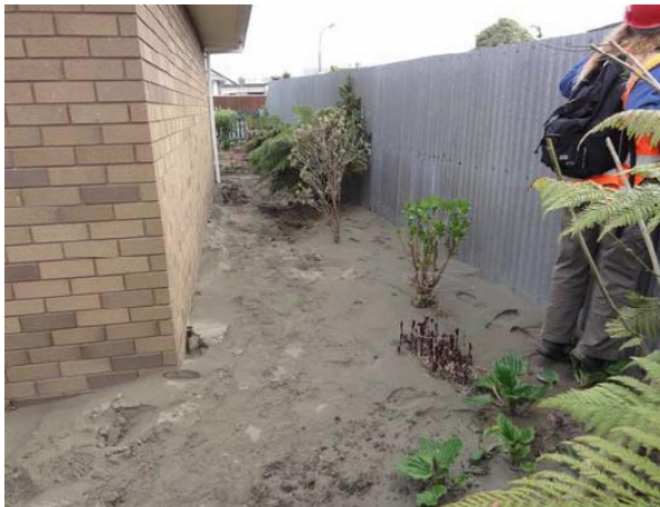
(a) Evidence of extensive liquefaction at the east end of Charles St.
