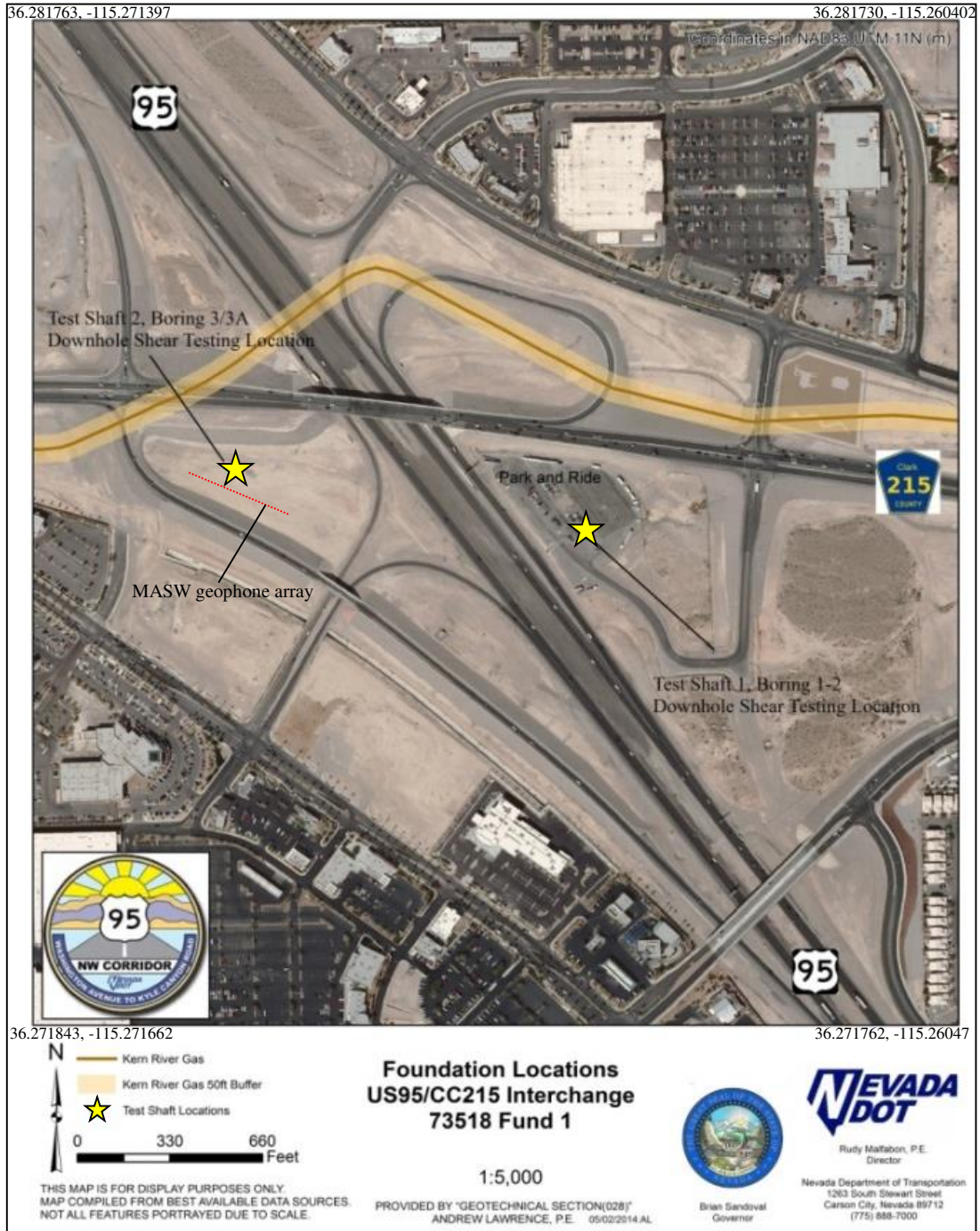
Figure 3.1: Vicinity of the borings and drilled load-test shafts at the US95/CC215 interchange; Hole 1 is denoted by ‘Test Shaft 1, Boring 1-2’ and Hole 2 is denoted by ‘Test Shaft 2, Boring 3/3A’.
