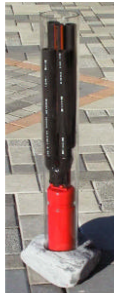
Photo 2. End of double U-tube BHE (Geowatt).
