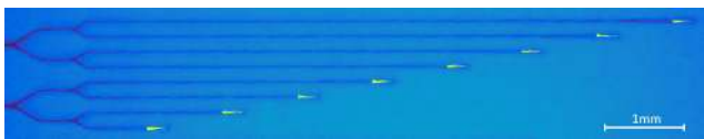
Fig. 9. Top view image of the waveguide loss section taken by a MIR camera.
