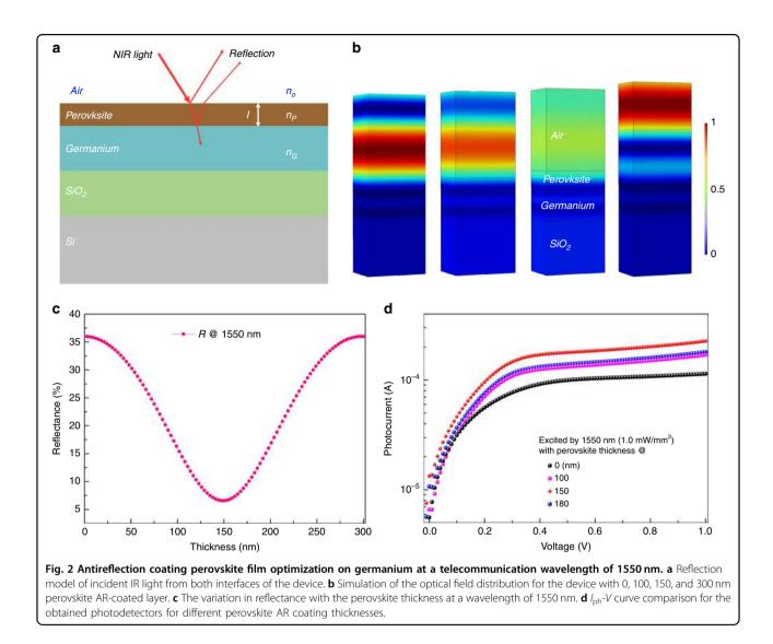
obviously in the perovskite AR-coated device. The highest  $I_{ph}$  value is obtained in a heterojunction device when the perovskite AR coating thickness is approximately 150 nm. The experimental results also match the theoretical predication discussed above. Figure S4 presents the  $I_{ph}$ -V comparison for the pristine germanium and AR coating optimized device. The higher  $I_{ph}$  of the perovskite/germanium heterojunction device is obvious.
